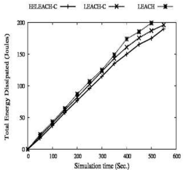
**Figure. 2.** Total Energy dissipated by all the nodes over time
