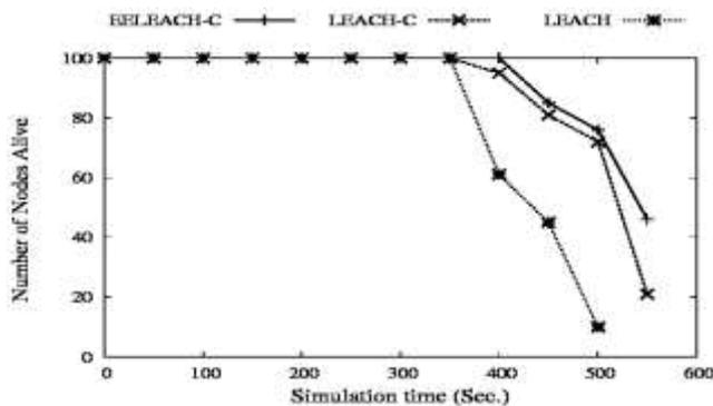
**Figure 4.** Comparison of LEACH, LEACH-C and EELEACH-C in terms of number of nodes alive
